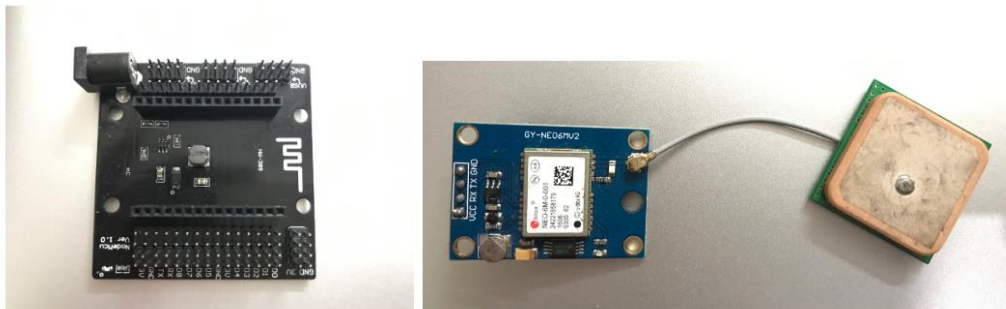
Fig. 14: (left)Breakout Board for NodeMCU with 12v supply support, (right) Ublox Neo6mv2 GPS device
